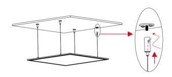
4. Steel wire rope though locker, then locker fixed with flat washer
